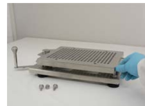
7. Secure with four thumb screws.
