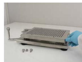
3. Unscrew 4 thumbscrews from corners of Filler Base.
