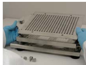
6. Position new size Body Sheet Set on Filler Base.
